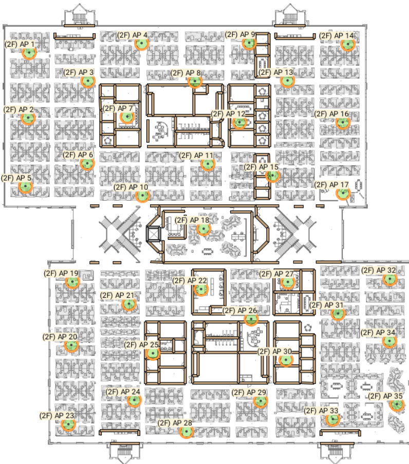
Example of floorplan with proposed access point locations based on active wireless survey
